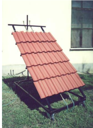
Fig. 4: The layout of a shell-structured solar collector
