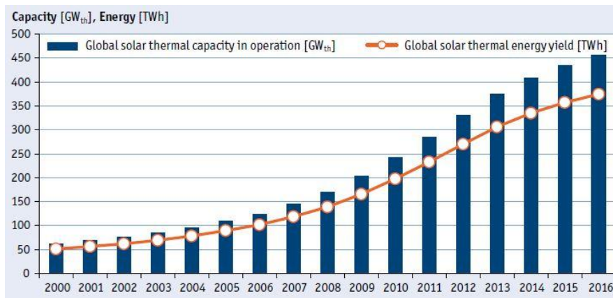
Fig. 3: Global solar thermal capacity in operation and energy yield for the period of 2000-2016
