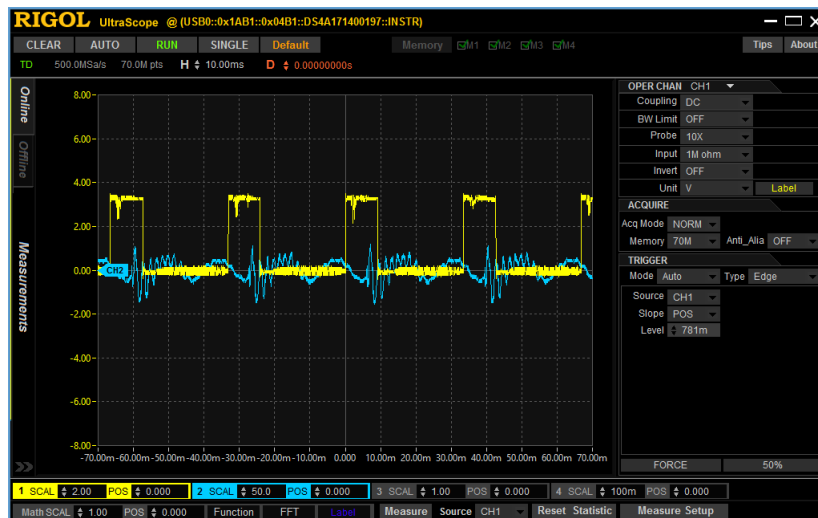
Fig. 11: Data Capturing from Oscilloscope with The Input Pulse 30 Hz
