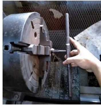
Figure 11. Making the Brushing Pipe
