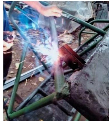
Figure 13. Making the Spring Bracket
