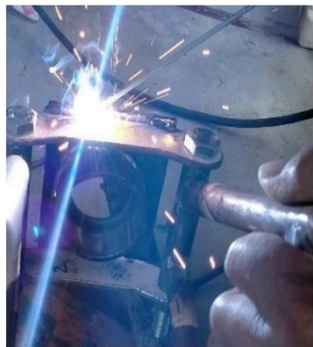
Figure 12. Making the Wheel Hub
