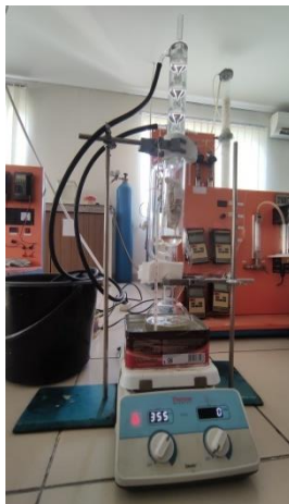
FIGURE 1. Coriander Seed Oil Extraction Process Soxhlet Extraction
