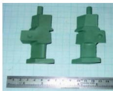
Fig. 3: Wax pattern of the injection results
