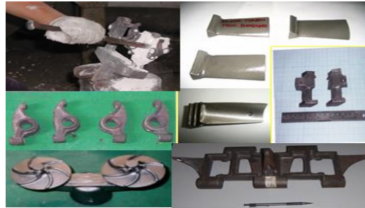
Fig. 5: Casting product results by using investment casting
