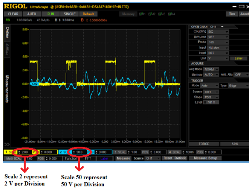
Fig 8. Data Capturing from Oscilloscope with The Input Pulse 91.24 Hz
